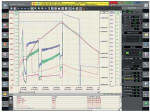
Process display and execution take place on a fully graphical interface (available in several languages) wherein the self-explanatory navigation is realized via touch-screen. Alphanumeric entries are carried out via an on-screen keypad. As an option, the plant can also be operated via mouse and keyboard.
